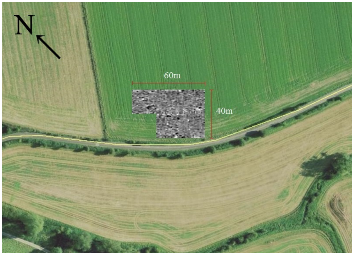
Fig. 6 The magnetometry results overlaid onto an aerial view of the survey area
