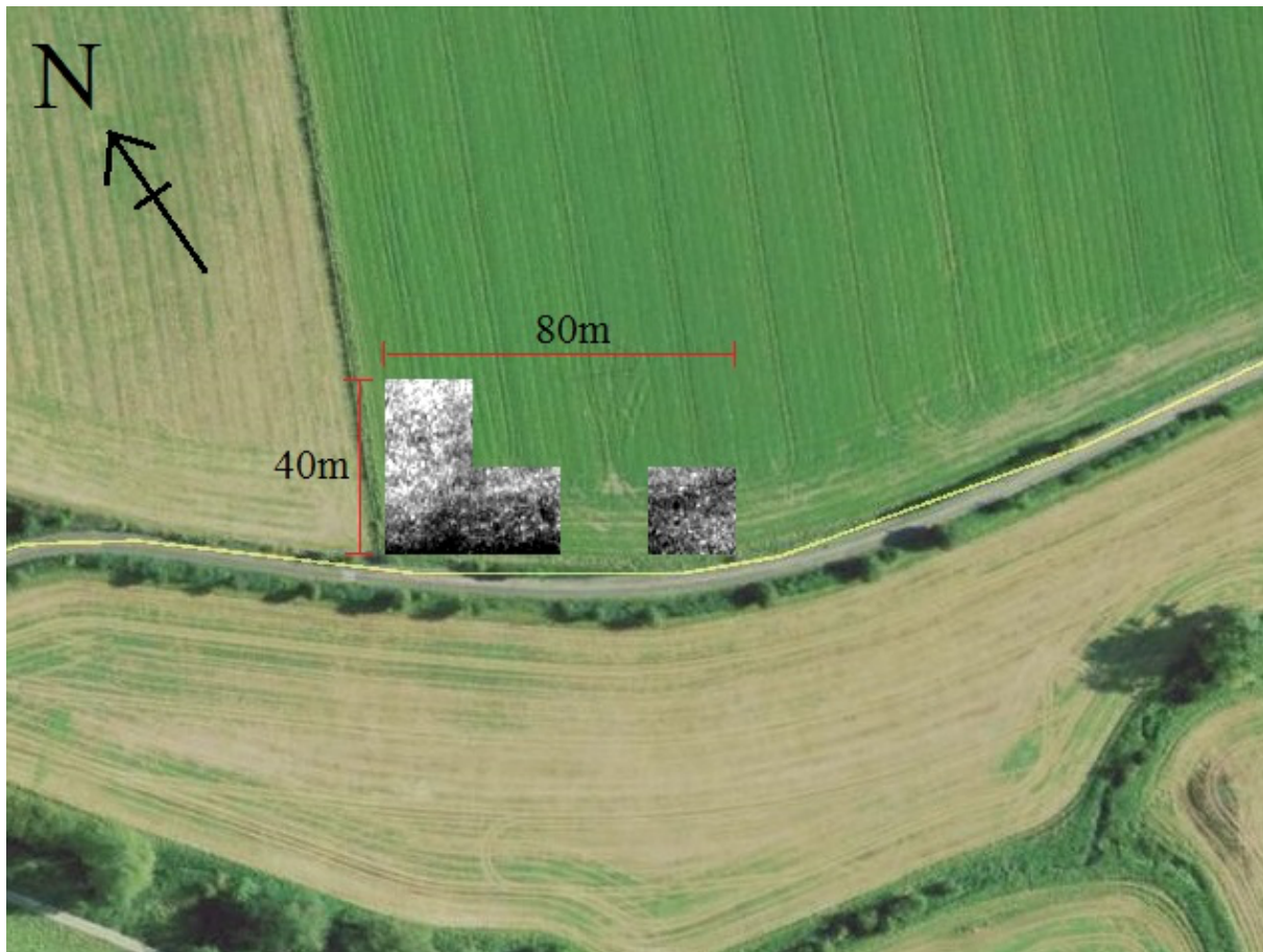
Fig. 7 The resistivity results overlaid onto an aerial view of the survey area
